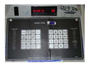
The "Old" Nevco controller is a larger unit than the newer ones. The connections for a remote start/stop switch are round 5 pin connectors (1980's PC keyboard type). The Run/Stop switch is located at the top left of the unit. It should be all the way up to Run, and all the way down to Stop. If a hand-held remote switch is connected, the Run/Stop switch on the unit should be placed in the middle position.
