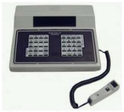
The "New" Nevco controller is slightly smaller than the older unit, has a slightly larger display and more features. The connections for a remote start/stop switch are on the side and are modular telephone type connectors. If a remote start/stop switch is not used, the start/stop buttons on the lower left of the keyboard should be used.
